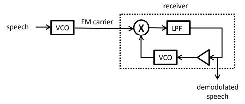
You will use two VCOs. For both of these VCOs, the mode should be set to "VCO" (on the PCB) and the toggle switch on the front panel should be set to "HI". Adjust the nominal frequency of each VCO to approximately 100 kHz. The sensitivity of each VCO should be adjusted to -1 kHz/V.
