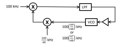
The feedback action of this loop will drive the VCO such that the difference frequency produced by the upper multiplier is zero. In other words, the loop (when in phase lock) will ensure that the two inputs to this multiplier have the same frequency.
